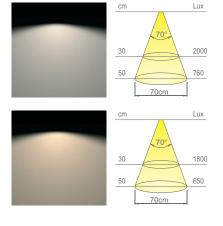
Colour temperature 4000 K 400 lm Luminous flux Luminous efficiency 80 lm/W CRI Ra ≥ 80 Colour appearance warm white Colour temperature 3100 K 375 lm Luminous flux Luminous efficiency 75 lm/W CRI Ra ≥ 80
