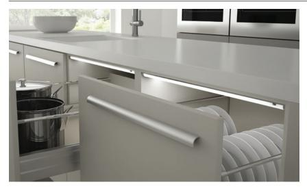
**LEAF DR** is a kitchen drawers and baskets LED profile with asymmetrical light projection. It is directly installed to the side of the cabinet's frame with concealed brackets and screws. The brackets allow for an application to the frame sides with a thickness of 16mm, 18mm and 19mm.
