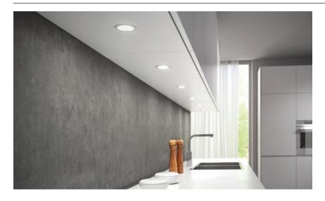
ATOM is designed for flush mounting with a Ø57mm hole and installation depth of only 8mm. It is installed in wooden panels with both through and blind holes. The fixing system, with two lateral springs, is quick and does not require any tool.
